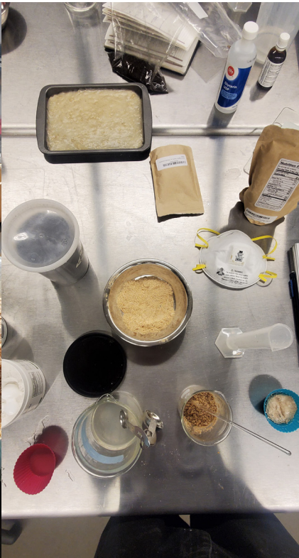
Making biocomposites in the BioLab using calcium carbonate, sodium alginate and sawdust
